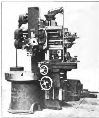
Fig. 4903. 36-Inch Boring and Turning Mill Fitted with Turret Head. Bullard Machine Tool Co.
